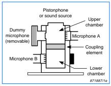
Fig.2 Simplified cross-section of intensity coupler
