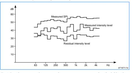
Fig.8 Sound intensity and mean sound pressure spectra measured in the field with an instrument calibrated with Type 3541. The residual intensity spectrum is obtained by subtracting the pressure-residual intensity index spectrum in Fig.7 from the measured SPL spectrum
