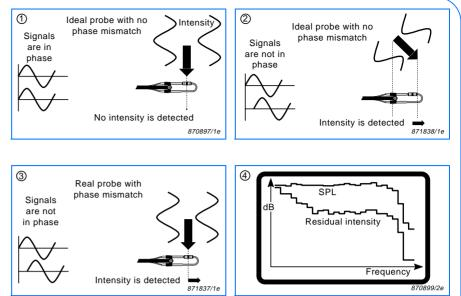
Even under controlled laboratory conditions, it is very difficult to create a free-field situation where the angle between the propagation of the sound wave and the probe axis is exactly 90 degrees (as shown in boxes 1 and 3). However, for practical applications this situation can easily be simulated using the set-up shown in Fig. 6.
