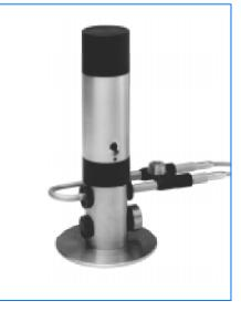
Fig. 6 Arrangement for measuring residual intensity and pressure-residual intensity index
