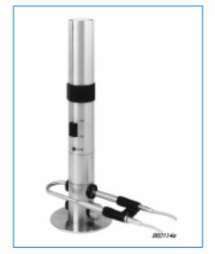
Fig. 4 Arrangement for sound pressure calibration
