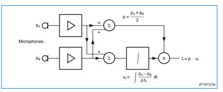
Fig.3 Simplified block diagram of an intensity measuring instrument. The signals from two pressure microphones,  $p_A$  and  $p_B$  are used to determine the pressure at the midpoint on the probe axis, p, and the particle velocity along the probe axis,  $u_r$ . Multiplying pand  $u_r$  gives the intensity reading  $I_r \Delta_r$  is the microphone spacing and  $\rho$  is the density of air
