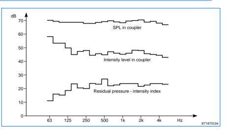
Fig. 7 Intensity and sound pressure levels measured with the arrangement shown in Fig. 6. The pressure-residual intensity index spectrum is characteristic of the measurement system and is obtained by subtracting these two spectra
